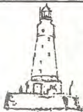
White Shoal Lighthouse. Black conical tower on sq. concrete pier, 360,000 cp Built 1910. . 118' ab. ground In the Straits of Mackinac at west end. 1929 lt. list.
